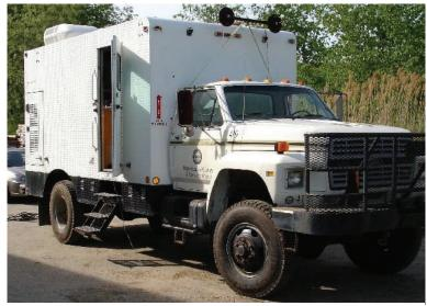
The WesternGECO-donated F700 seismic recording truck allows recording of up to 3000 channels of 24-bit digital data simultaneously. It has a 24 kV or can be run via shore power.
