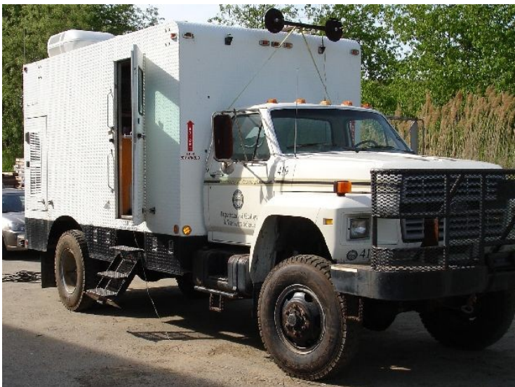
The WesternGECO-donated F700 seismic recording truck allows recording of up to 3,000 channels of 24-bit digital data simultaneously.
