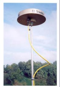
New University of Pittsburgh Seismic Station Second Picture: New CORS (continually operating recording station) GPS base station being run in cooperation between the National Geodetic Survey, PennDOT and G&PS.
